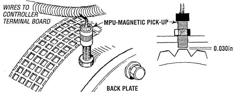
**NOTE:** If replacing the Magnetic Pick-Up (MPU) it **MUST** be replaced without cutting and splicing into the existing wiring cable. Doing so will cause a erratic AC signal to the controller.
